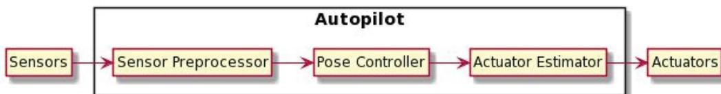
However, this barebones architecture is only able to control our aircraft to a fixed pose and only if already in flight and in similar conditions to the desired pose.
