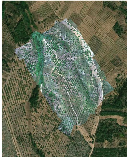
*orthophoto: merging the multispectral camera bands*
