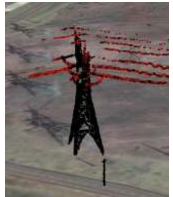
Figure 3 - the same tower with 3D point cloud over 2D surface modelled photo on a GIS (GoogleEarth™).
