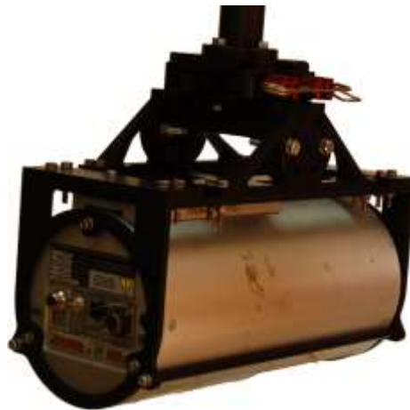
Figure 4 - ASLMS with a quick-release helicopter mount
